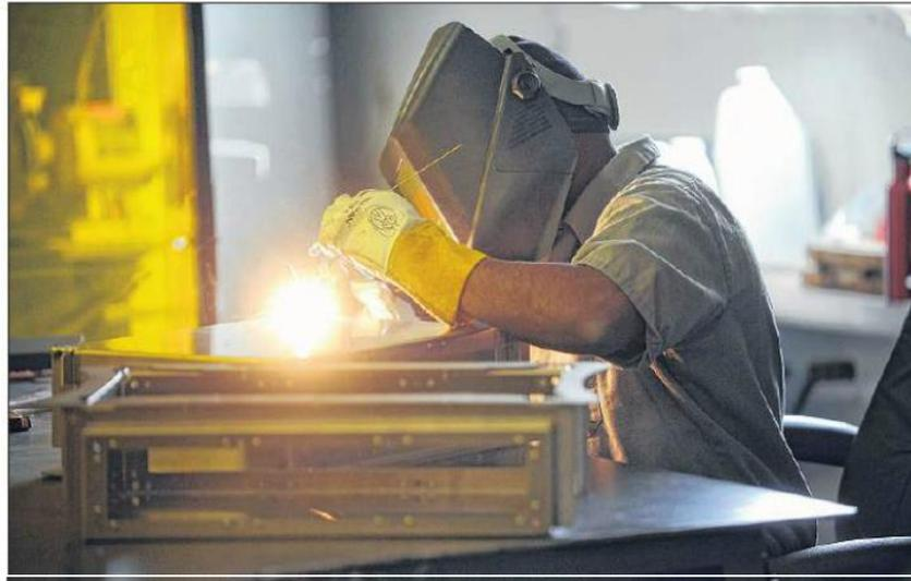
Jonathan Charles welds aluminum enclosures that will hold inverter boxes for solar panels at Metcam, a fabricator of custom sheet metal components and assemblies, in Alpharetta. BITA HONARVAR / AJC
